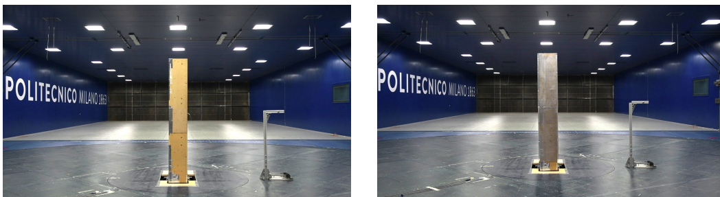
Figure 1. Comparison between the front view of the model without (naked) and with the mesh (PDSF).
