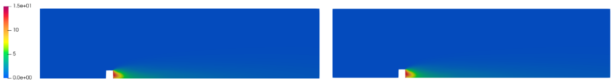
Figure 4. The pollutant concentration predicted by CFD simulation (left) and ROM simulation (right)
