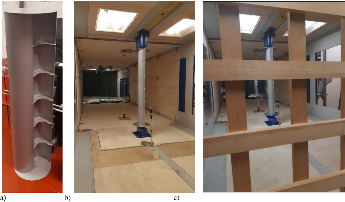
Figure 1. Savonius rotor (a), model in the wind tunnel with the generator and hot-wire anemometers (b); the wooden grid for turbulence generation (c)
